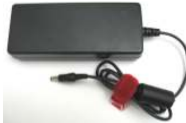
2. Power Supply unit (PSU) If you order a high-current supply, you should still receive a "stock" 65w/24v supply suitable for near-field listening or burn-in. We advise that you keep this on-hand for testing as well should you experience any challenges with your high-current supply.
